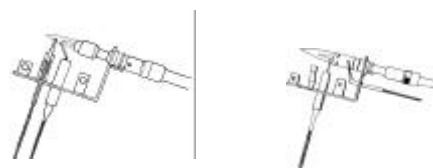
Fig 11 NATURAL GAS ODS PILOT LIQUID PROPANE ODS PILOT
